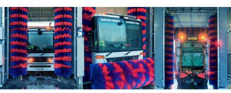
Cleaning is achieved by applying a diluted detergent solution directly to the exterior of the vehicle while simultaneously scrubbing with rotating brushes. This process is then repeated, without detergent to rinse the vehicle clean.
